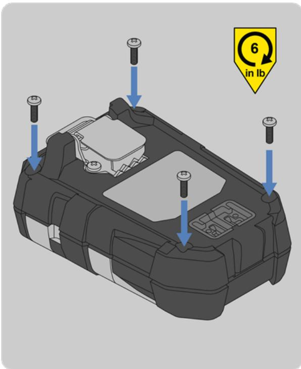
7. Install the four external screws with a Phillips head #1 torque screwdriver. Torque to 6 in-lbs (0.68 N-m).
