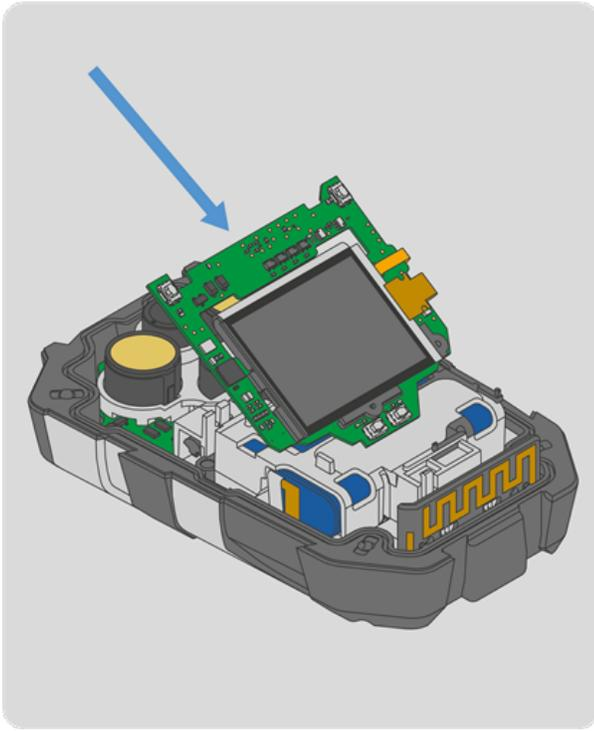
9. Take the display PCBA and display assembly, and insert the bottom left edge under the snap fit on the battery holder. Push the display PCBA down to engage the board to board connector.
