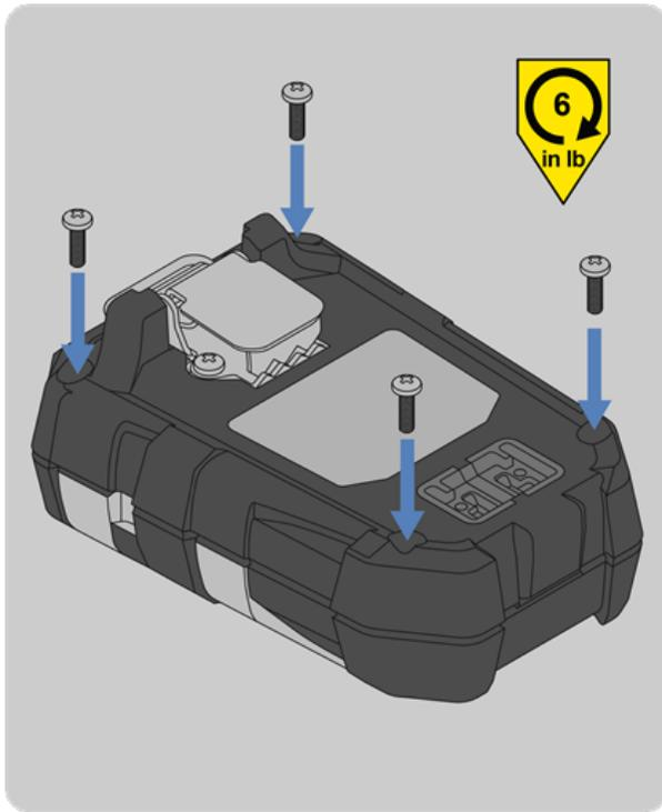
11. Install the four replacement screws with a Phillips head #1 torque screwdriver. Torque to 6 in-lbs (0.68 N-m).
