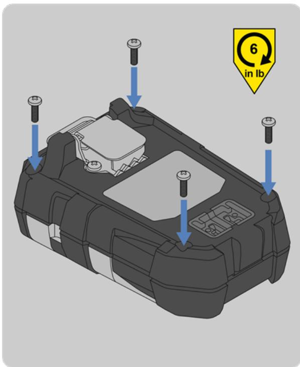
8. Install the four external screws with a Phillips head #1 torque screwdriver. Torque to 6 in-lbs (0.68 N-m).
